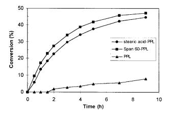
**Figure 1** Formation of 1-phenylethyl acetate with time by modified PPL. Experimental conditions were 10 mg protein, 50 mM 1-phenyl ethanol, 150mM vinyl acetate, 10 ml diisopropyl ether, with shaking at 35°C.
